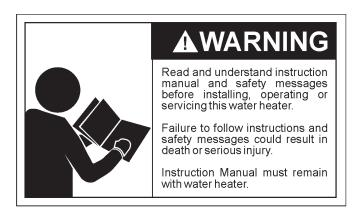
Read this manual first. Then before checking the water heater make sure the gas supply has been turned "OFF", and never turn the gas "ON" before the tank is completely full of water.
